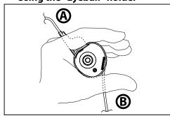
The HMH-100 is most effective when used with the "Eyeball" holder due to the close proximity of the microphone to the Harmonica.
