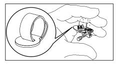
The lavalier clip can also be used with the hook and loop fastener attached to your finger as shown in the above illustration. This avoids accidental dropping of the microphone when the hand has opened.
