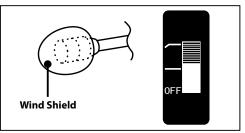
We recommend using the included wind shield (pop filter) with your HMH-100 microphone to reduce wind noise. It is also possible to reduce wind noise by setting the switch to the " / " position which cuts low frequency.
